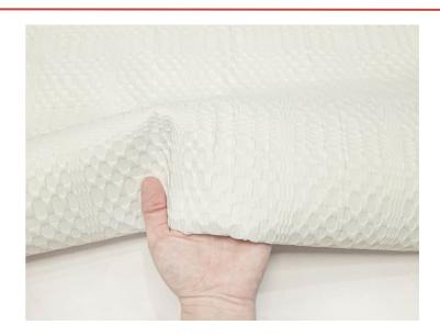
**Jacquard fabric** is characterized by the design being woven into the fabric, creating a raised pattern with incredible texture, which woven types of Weaving and Knitting.
